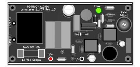
This power supply is designed to drive traditional neon as well as other gas filled displays using 1 or 2 electrodes. With the onboard PWM adjustment knob, the display can be dimmed from full on to almost completely off while maintaining an even intensity throughout the tube. The PWM adjustment also provides control over the plasma discharge in single electrode displays allowing for additional creativity and experimentation.
