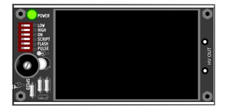
This power supply is designed for 2 electrode traditional neon units. Using the small DIP switches located on the power supply, you can select 1 of 4 different operating modes, FLASHING, SCRIPTING, PULSING and STEADY. The rate/ speed of the effect is adjusted with the speed knob located next to the DIP switches as well as a low/high range selected by the DIP switches.
